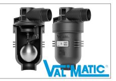
The Val-Matic Resilite Combination Air Valve has been designed to meet the performance requirements of AWWA Standard C512 and to be used with clean water. Each valve features corrosion resistant materials of construction, full-ported flow area maintained throughout, NPT threaded connections, stringent testing, and NSF 61 Certified.
