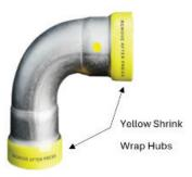
The yellow shrink wrap hubs will fall off after pressing, providing visual confirmation that the fitting has been pressed. If it does not fall off, then you may have to remove it by hand.
