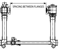
**Prior to and during installation,** verify flange-to-flange spacing required for meter and gaskets to ensure proper installation. Spacing may have been altered during shipment or installation.
