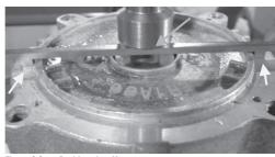
Figure 2 Gage Positioned on Motor (PICTURED WITHOUT PUMP END)
