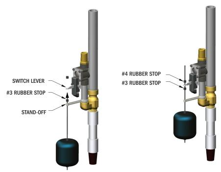
4. Loosely attach the pump mount clamp to the 1¼" discharge pipe of the pump.
