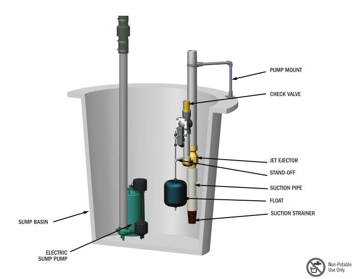
WARNING Sump water is non-potable. To reduce the risk of contamination of the potable water supply, this pump must be installed with a listed backflow prevention device suitable for the installation, in accordance with the local plumbing code, such as a reduced pressure zone backflow preventer (RPZ). Alternatively, consult the local plumbing and health codes or the authority having jurisdiction for guidance on cross-connection and backflow protection requirements.
