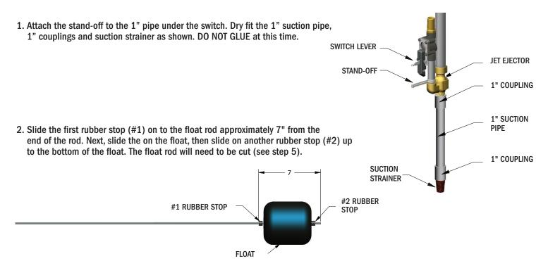
3. Insert the float rod into the stand-off hole. Slide on rubber stop (#3) 8" from the top of the rod. Slide the float rod through the hole in the lever. Then slide on rubber stop (#4) 1" above rubber stop (#3).
