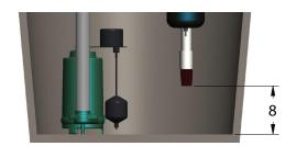
Position the Guardian assembly over the sump basin where the suction strainer is roughly 8" from the bottom of the basin. In some shallow basins the 1" suction pipe may need to be cut.
