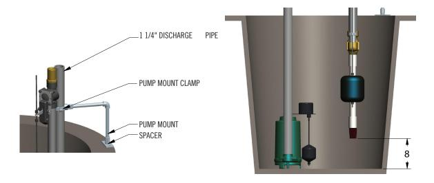
Position the Guardian® assembly over the sump basin where the suction strainer is roughly 8" from the bottom of the basin. In some shallow basins the 1" suction pipe may need to be cut.
