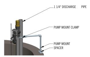
The float rod must easily move up and down and be in the vertical position. Make sure the float does not interfere with the electric sump pump, power cord or side of the basin.
