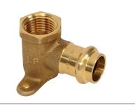
A.Y. McDonald Mfg. Co. No-Lead Drop Ear Elbows creates a 90° connection and allows the transition from Pex tubing to threaded pipe. Drop ear elbows are secured to a stud behind the wall, using the mounting 'ears' which have holes in them. Typically used for installing shower arms and tub spouts, and for use in potable water applications.
