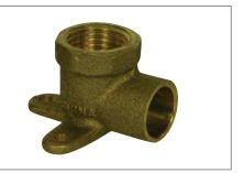
A.Y. McDonald Mfg. Co. No-Lead Drop Ear Elbows creates a 90° connection and allows the transition from Pex tubing to threaded pipe. Drop ear elbows are secured to a stud behind the wall, using the mounting 'ears' which have holes in them. Typically used for installing shower arms and tub spouts, and for use in potable water applications.
