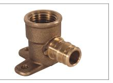
A.Y. McDonald Mfg. Co. No-Lead Drop Ear Elbows creates a 90° connection and allows the transition from Pex tubing to threaded pipe. Drop ear elbows are secured to a stud behind the wall, using the mounting 'ears' which have holes in them. Typically used for installing shower arms and tub spouts, and for use in potable water applications.
