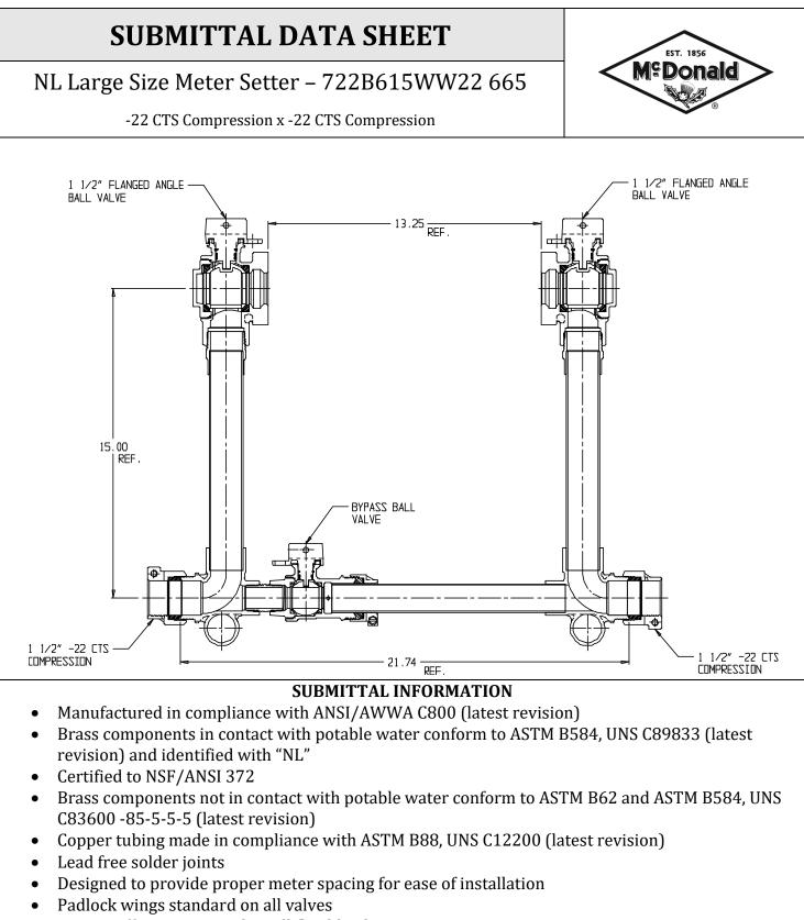
• Insert stiffeners required on all flexible plastic connections
