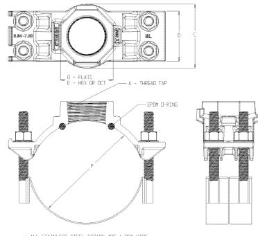
\*\* ALL STAINLESS STEEL STRAPS ARE 1.88" WIDE. TWO STRAPS (WITH 2 STUDS WELDED ON) PER ASSEMBLY.
