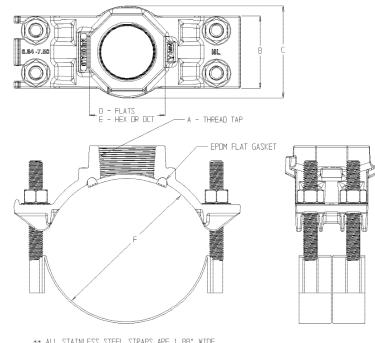
\*\* ALL STAINLESS STEEL STRAPS ARE 1.88" WIDE. TWD STRAPS (WITH 2 STUDS WELDED DN) PER ASSEMBLY.
