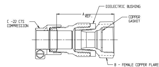
NDTE: ACTUAL LENGTHS WILL VARY DUE TO ASSEMBLY DF INSULATOR.
