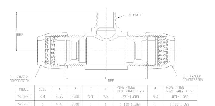
NDTE: McDDNALD RANGER NUTS ARE NDT COMPATIBLE WITH DTHER MANUFACTURERS COMPRESSION NUT SYSTEMS McDDNALD RANGER NUTS ARE NDT COMPATIBLE WITH DTHER McDDNALD COMPRESSION NUT SYSTEMS
