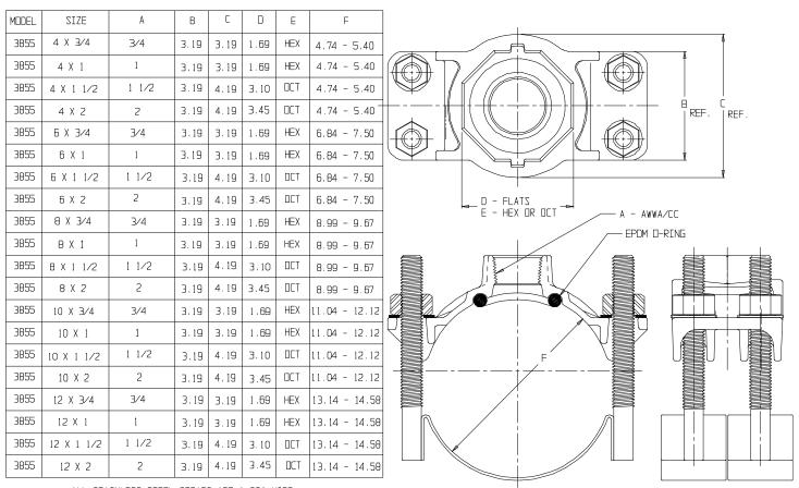
\*\* ALL STAINLESS STEEL STRAPS ARE 1.88" WIDE, TWD STRAPS (WITH 2 STUIR VELOCIAL ON ) PER ASSEMBL
