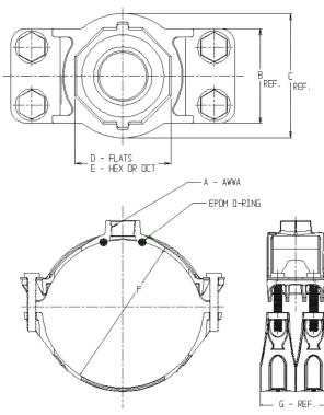
\*\* ALL 85 BRASS STRAP. TWO STRAPS PER ASSEMBLY. DRAWING MAY NOT RESEMBLE ACTUAL SADDLE CONFIGURATION
