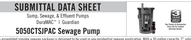
This pre-assembled simplex sewage package is designed to be used in any residential sewage application. With a 30 gallon capacity, 2" solids handling, and a 2" discharge pipe connected to the sewage pump, the package is ready to be installed.
