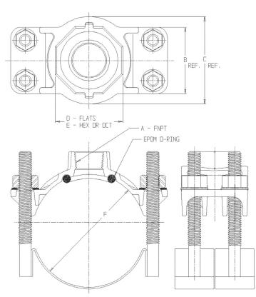
\*\* ALL STAINLESS STEEL STRAPS ARE 1.88" WIDE. TWO STRAPS (WITH 2 STUDS WELDED ON) PER ASSEMBLY.
