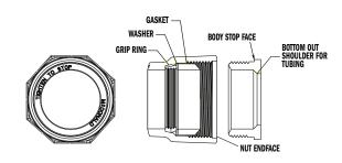
The A.Y. McDonald McGrip "G" & "-3G" Series compression system is a simple convenient method of connection for tube size service materials
