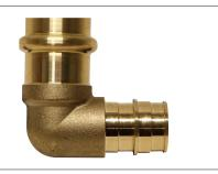
A.Y. McDonald Mfg. Co. copper press fittings are for use in plumbing or mechanical applications. Sizes range from 1/2" - 1" and the fittings are designed to join ASTM B88 (Types K, L, M) hard-drawn copper tube and soft copper tube on the press end and PEX Tubing in accordance with ASTM F876 & F877 on the PEX end.
