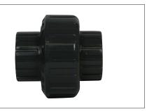
A.Y. McDonald Mfg. Co. PVC Fittings feature convenience of operation with excellent flow characteristics. A PVC union is used to join two pieces of pipe. Unlike couplings, unions use a gasket seal to create a removable connection between pipe.
