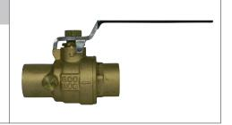
A.Y. McDonald Mfg. Co. No-Lead Ball Valves with drain are constructed from heavy duty no-lead brass They are designed for residential and commercial use on steam, oil, water or gas. The full port allows for maximum flow, minimum pressure drop and turbulence. The drain feature allows for drainage of water down line to prevent freeze up.
