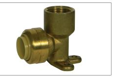
A.Y. McDonald Mfg. Co. No-Lead Drop Ear Elbows creates a 90° connection and allows the transition from Pex tubing to threaded pipe. Drop ear elbows are secured to a stud behind the wall, using the mounting 'ears' which have holes in them. Typically used for installing shower arms and tub spouts, and for use in potable water applications.
