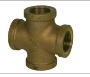
A.Y. McDonald Mfg. Co. No-Lead Pipe Fittings & Nipples are constructed from heavy duty bronze and are rated for commerical, industrial and residential applications up to 125 WOG. Threads conform to ANSI B1.20.1 and fitting dimensions comply with ANSI B16.15.
